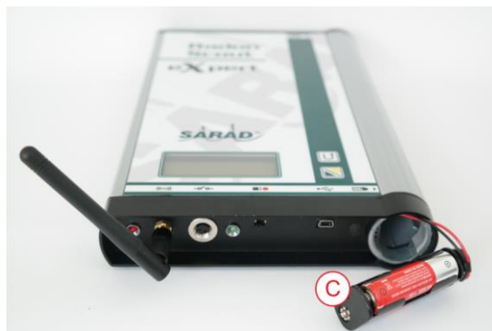
Fig. 5. – Replace the batteries (C). Take care for right polarity.
