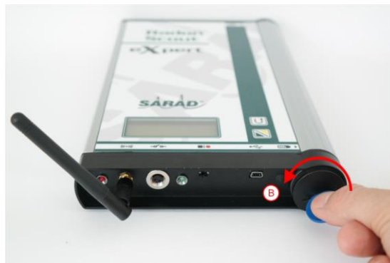
Fig. 4. – Unscrew the battery cover (B) at the side panel.
